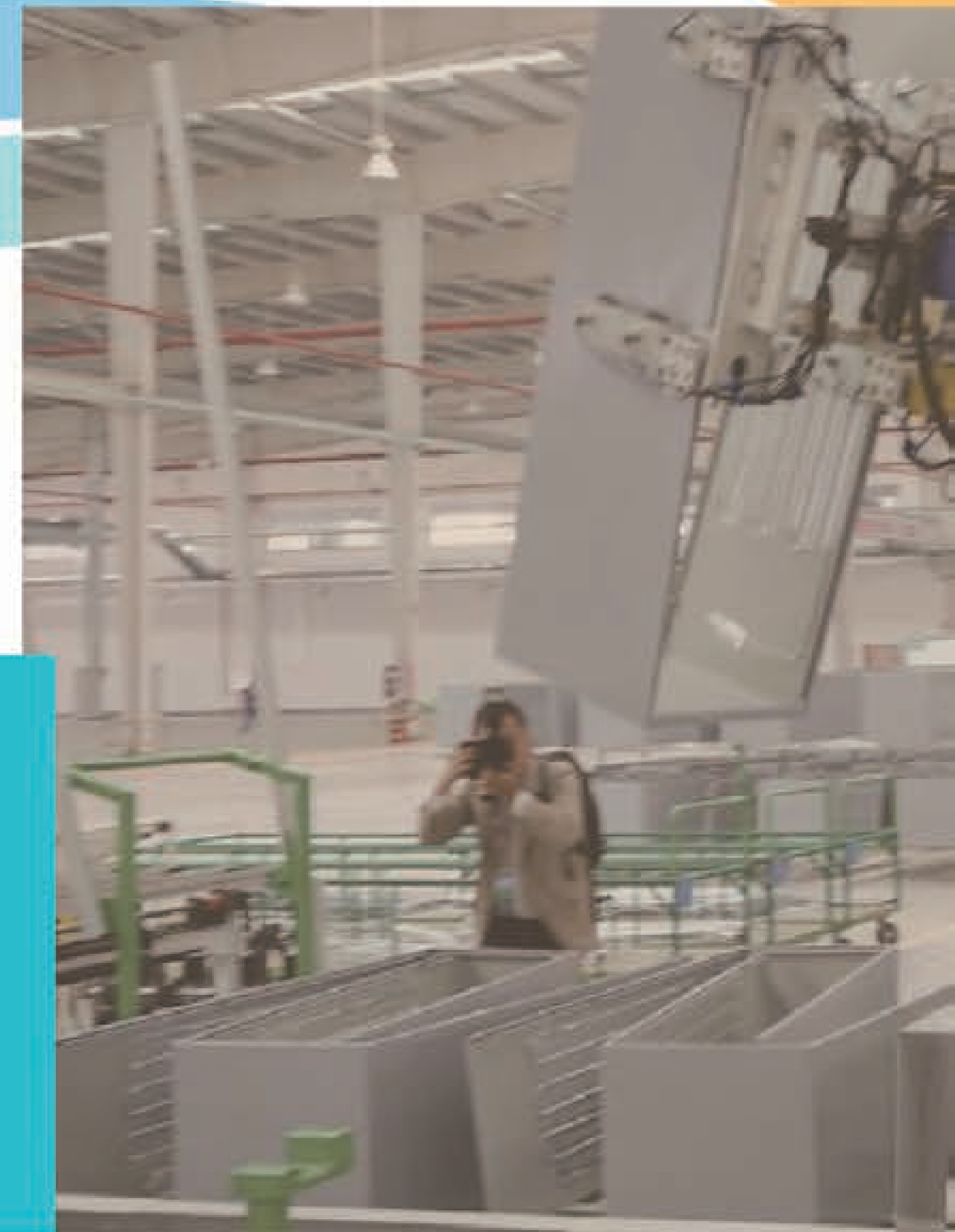
Robot arm takes U-shaped shell from the assembly line
